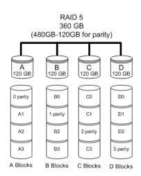
Figure 3. RAID 5 Configuration Example
